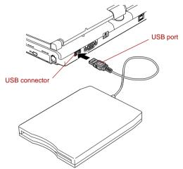
Figure 3-27 Connecting the USB floppy diskette drive
